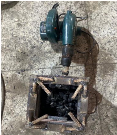
Fig. 4. Charcoal Pot incorporated with a Blower
