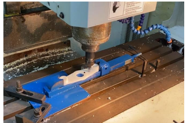
Fig. 6. Proof-of-concept milling trial with a polymer linkage bracket.
