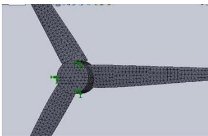
Fig. 15. Wind turbine after creating the mesh
