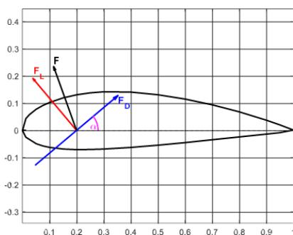
**Fig. 3. Angle of Attack**
