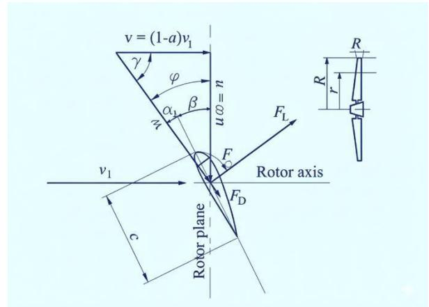
**Fig. 4. Velocities and angles of the wind turbine**
