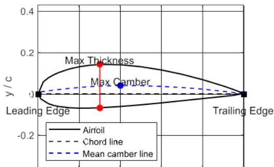
**Fig. 2. Airfoil geometry with key parameters**
