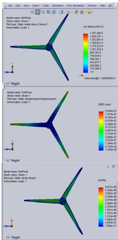
Fig. 15. Static simulation results
