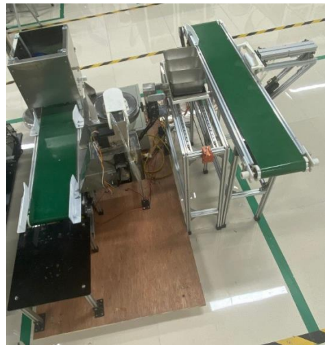
Fig. 13. The completed prototype of the automatic tray feeding modul
