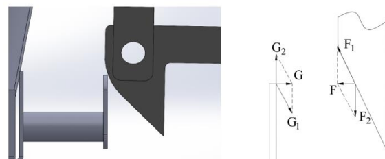
Fig. 10. Force diagram of the hook and tray mechanism
