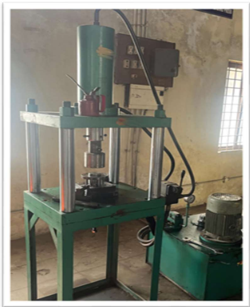
Figure 12 Deep drawing machine with hydraulic-powered press
