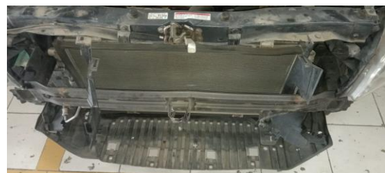
Fig. 2 Car Frontal Crush Can Assembly
