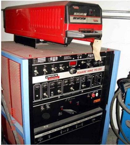
Fig. 1 Square Wave TIG 355 Welding Power Source
