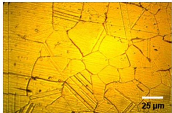
**Fig.1 Optical microstructure of C263 nickel based super alloy**
