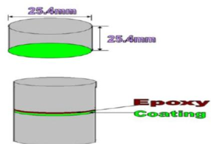
Fig. 5 Specimen for Tensile bond strength
