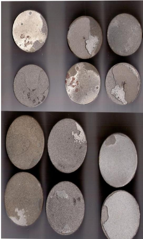
Fig. 6(b) Coated Specimen after bond test
