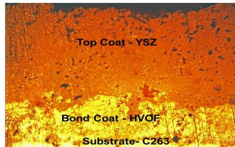
Fig. 9 Microstructure of YSZ coating with BC
