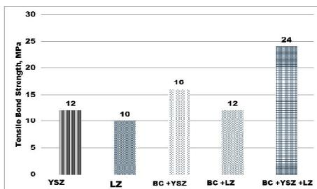
Fig. 12 Comparison of Bond strength values of different coating architecture
