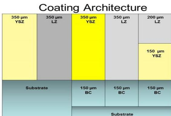
Fig. 4 Coating architecture for Bond strength
