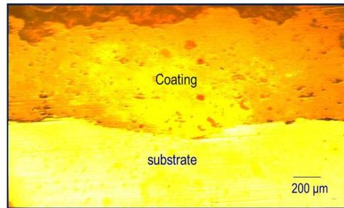
Fig. 7 Microstructure of YSZ coating without BC
