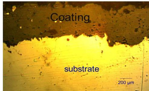
Fig. 8 Microstructure of LZ coating without BC
