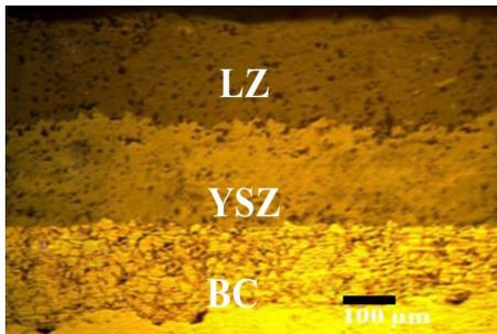
Fig. 11 Microstructure of Double Ceramic layer coating
