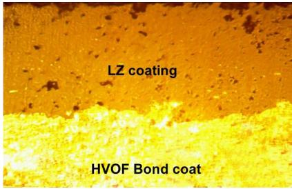
Fig. 10 Microstructure of LZ coating with BC
