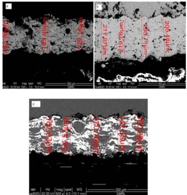
**Fig. 3 Thicknesses of the Coatings (a) WC-Co (b) NiCrBSi (c) WC-Co+NiCrBSi**
