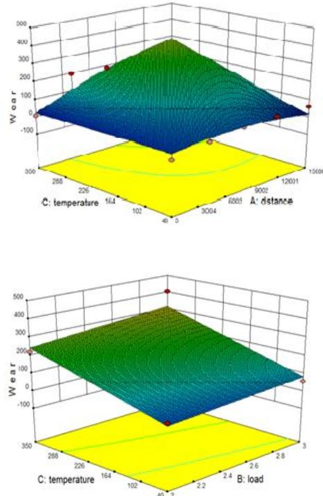
**Fig. 5(f) 3D graphs showing the interaction effect of different parameters for WC-Co +NiCrBSi Coating.**
