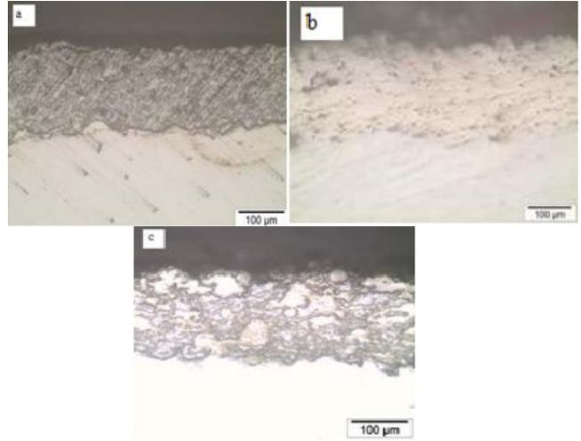
**Fig. 2 Microstructure of Coatings (a) WC-Co (b) NiCrBSi (c) WC-Co+NiCrBSi**
