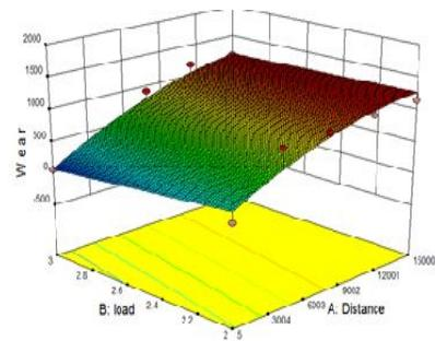
Fig. 5(b) 3D graphs showing the interaction effect of different parameters for WC-Co Coating
