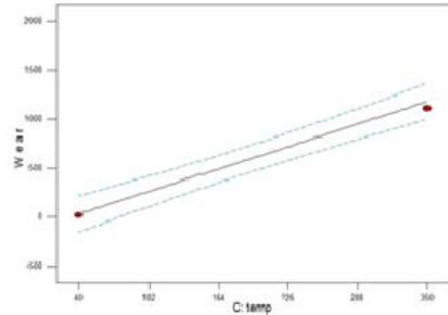
Fig. 5(c) Graphs showing the variation of wear with respect to single parameter for NiCrBSi Coating
