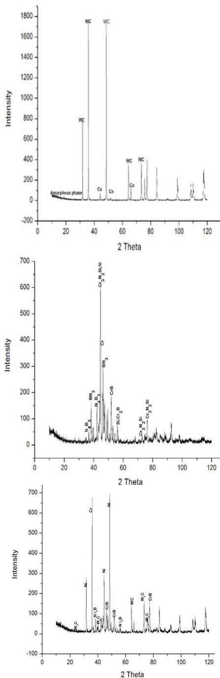
Fig. 4 XRD of the Coatings (a) WC-Co (b) NiCrBSi (c) WC-Co+NiCrBSi
