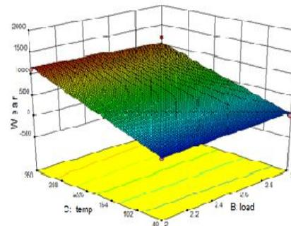
Fig. 5(d) 3D graphs showing the interaction effect of different parameters for NiCrBSi Coating
