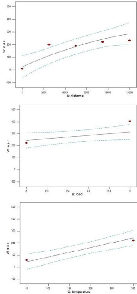
**Fig. 5(e) Graphs showing the variation of wear with respect to single parameter for WC-Co+NiCrBSi Coating**
