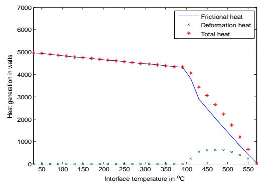
**Fig. 4 Heat generation due to friction, deformation and total as a function of temperature for 900 rpm**
