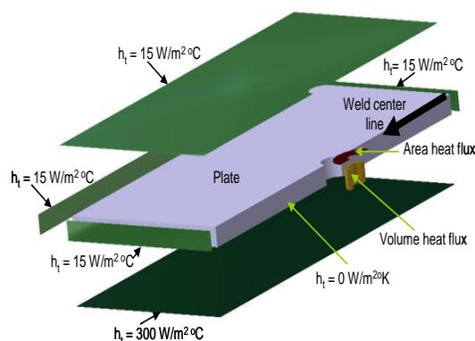
Fig. 2 Finite element model with heat inputs and boundary conditions
