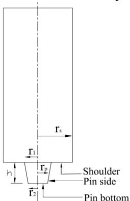
Fig. 1 FSW tool dimensions
