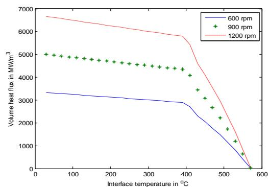
**Fig. 5 Volume heat flux at the pin for 600, 900 and 1200 rpm**
