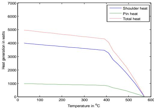
**Fig. 3 Heat generation at shoulder, pin and total as a function of temperature for 900 rpm**
