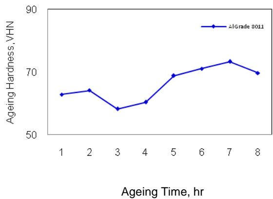
Fig. 9 Effect of ageing temperature at 190° C on Hardness of Al 8011
