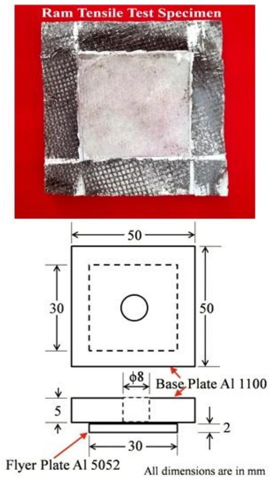
**Fig: 2 Ram Tensile Test Specimen with dimensions.**
