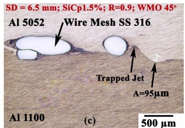
Fig. 4 Microstructure of Al-Al explosive clad.
