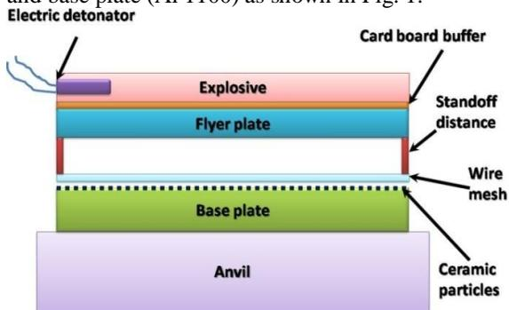
**Fig. 1 Parallel configuration Explosive Cladding.**
