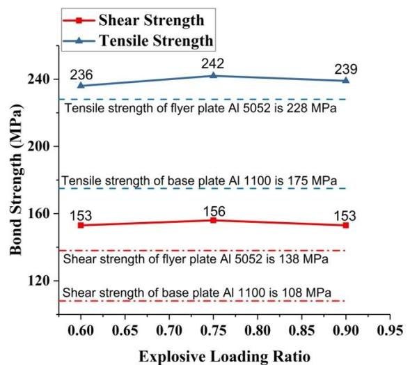
**Fig. 6 Bond strength of explosively clad plates measured by the tensile and shear test.**
