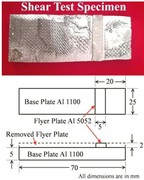
Fig. 3 ASTM Side Shear Test Specimen with dimensions.
