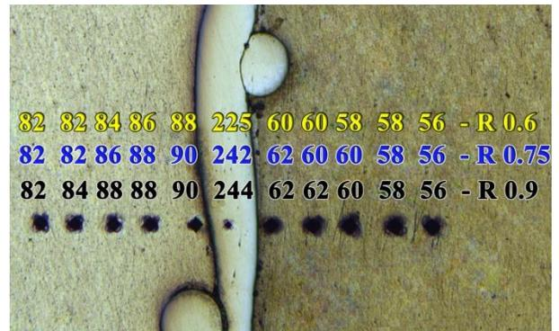
**Fig. 5 Vickers Hardness variation across the interface**
